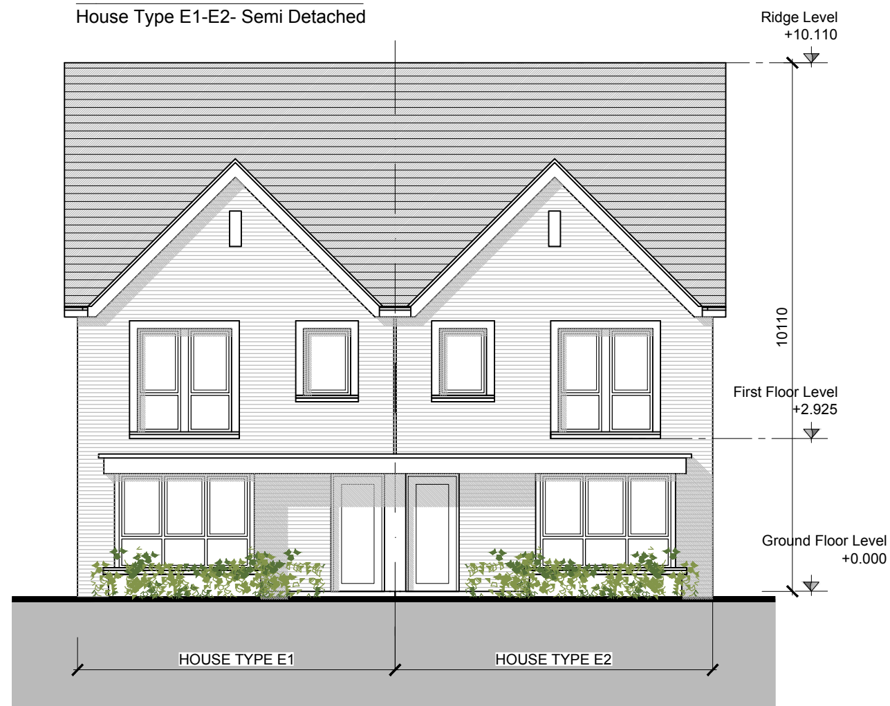
FRONT ELEVATION House Type E1-E2- Semi Detached
